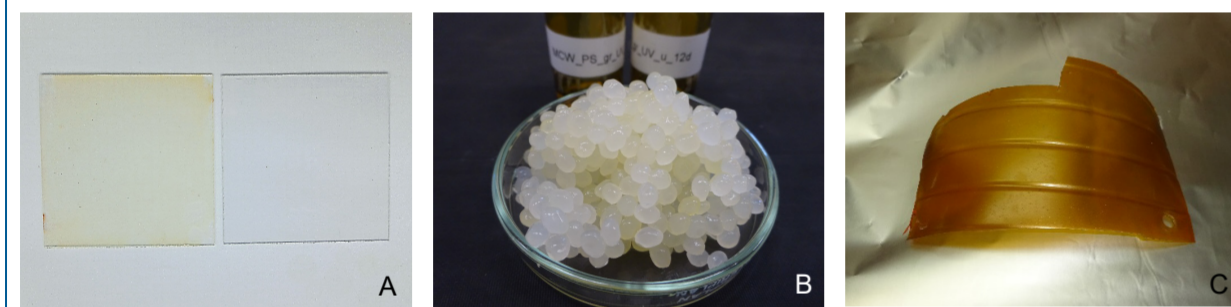
Figure 1: Samples of different polymers (Low density polyethylene (LDPE), Polystyrene (PS), and Polyethylene terephthalate (PET)) were used as sheets (A), granulates (B), and bottle fragments (consumer product, C).
